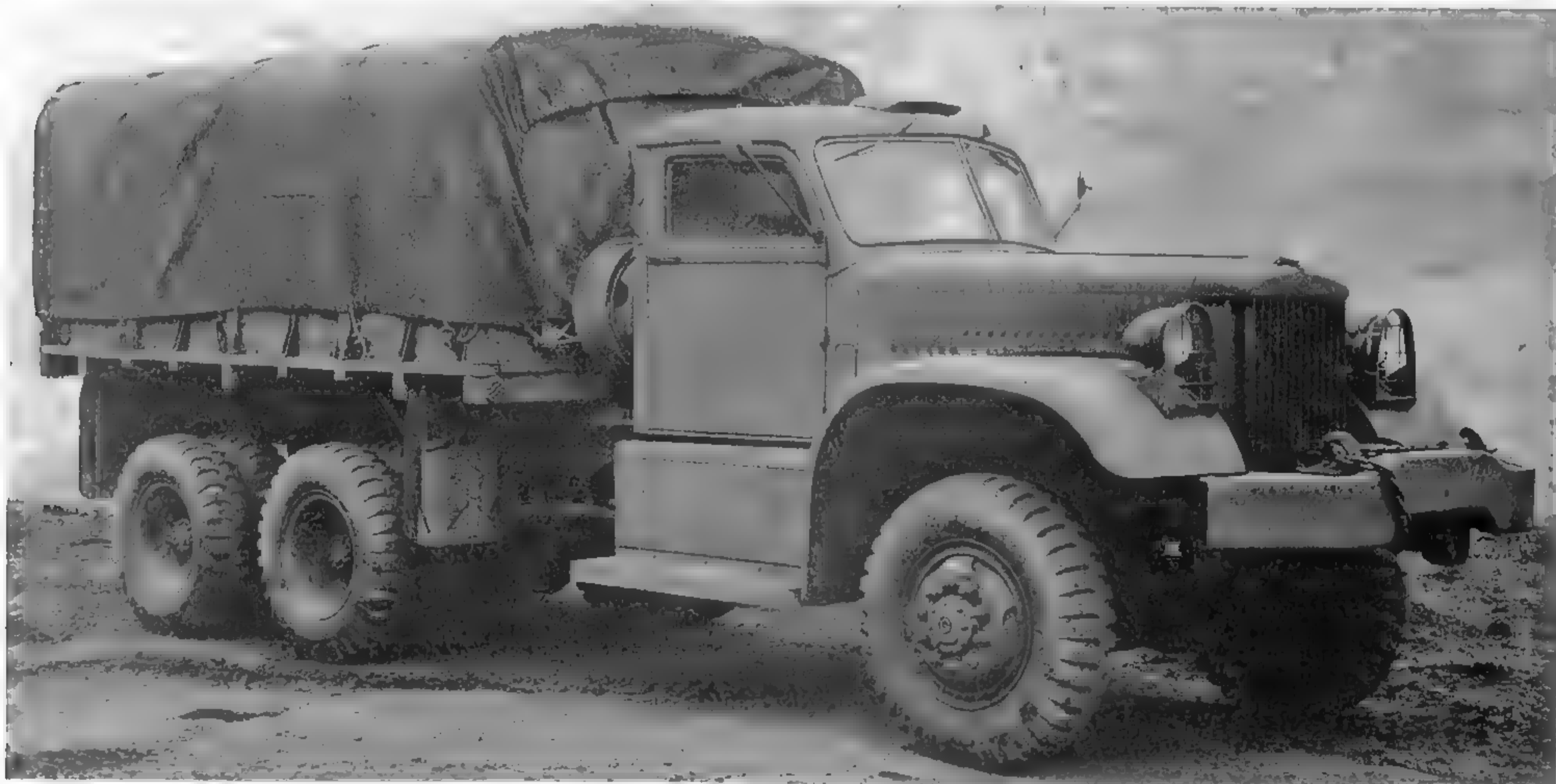
Seen in this view of the same truck are the other spare wheel, the liquid container and its rack, and cargo canvas. The lead chain for the front winch can be seen wrapped around the bumper. Notice that the bed is wooden, but has the King Bee reflectors. (U.S. Army photo)
